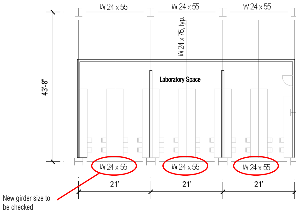
Typical Wet Lab Floor Plan (superimposed onto framing plan):
